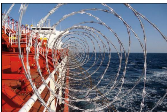
Barbed wire on the gunwale of a merchant ship to prevent pirate boardings / MARFLET
